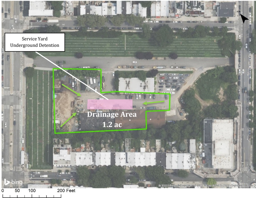
Figure 12: Practice 1 - Service Yard Underground Detention Drainage Area
